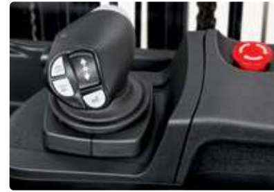
Optional joystick with integrated controls
